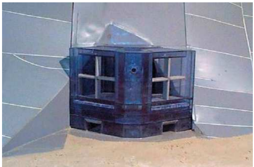
Intake structure, hydraulic model
