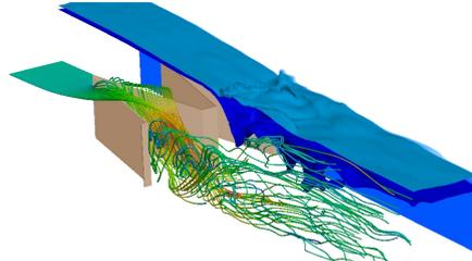
FIG. 3. WATER FLOW IN A SPILLWAY
