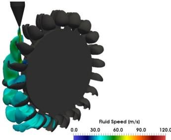
FIG. 1. WATER FLOW IN PELTON TURBINE
